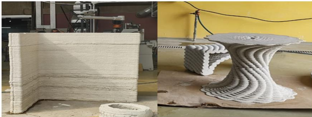
Figure 2 – Kitchen walls and construction of utensils using a 3D printer
